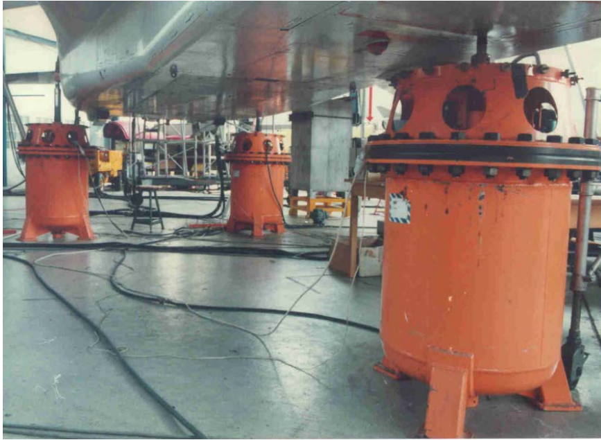
Figure 9: Air spring system used for Ground Resonance Tests
