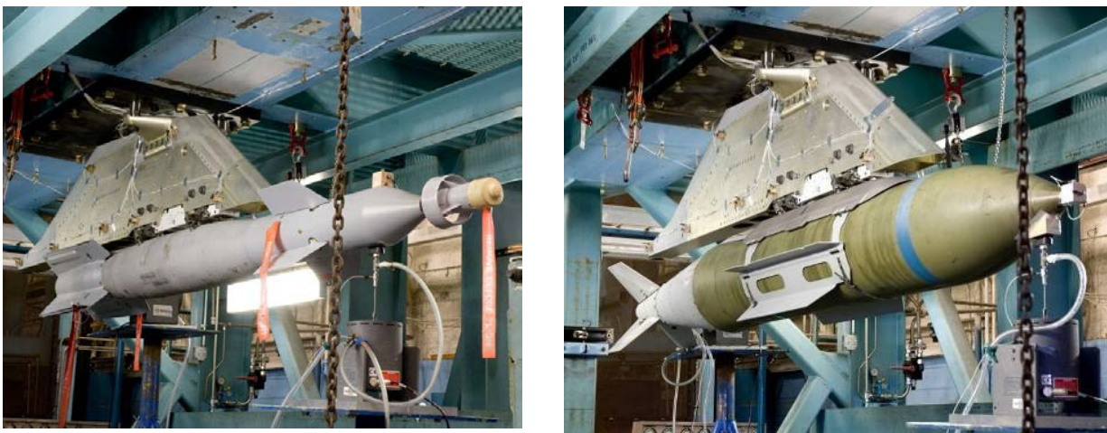
Figure 8: Fixed component Ground Vibration Test with different stores, courtesy of Lockheed Company
